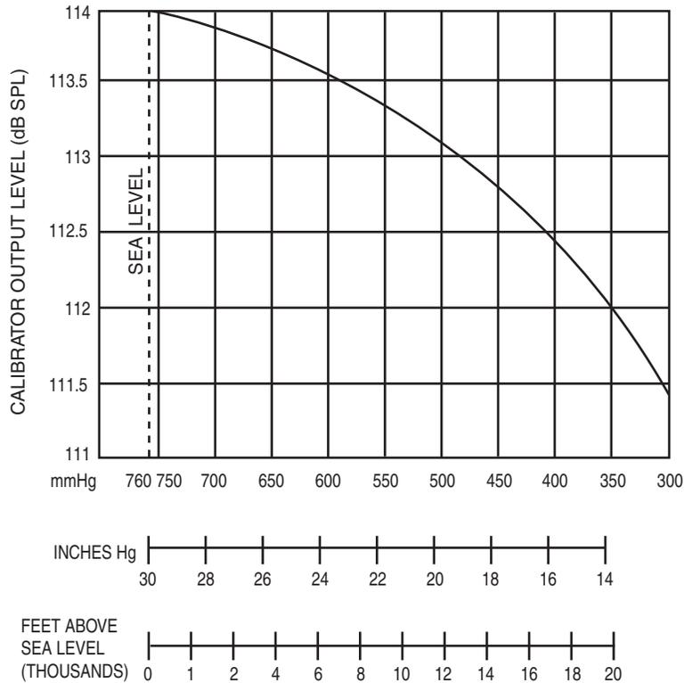
Figure 3-2. Effect of Elevation Upon Calibrator Output
