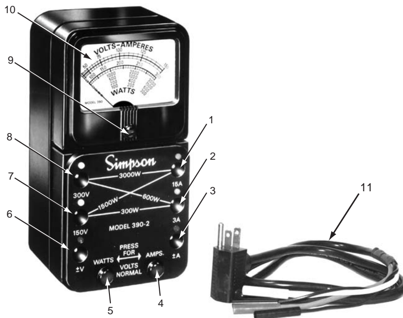
Figure 3-1. Controls, Connectors and Indicator
