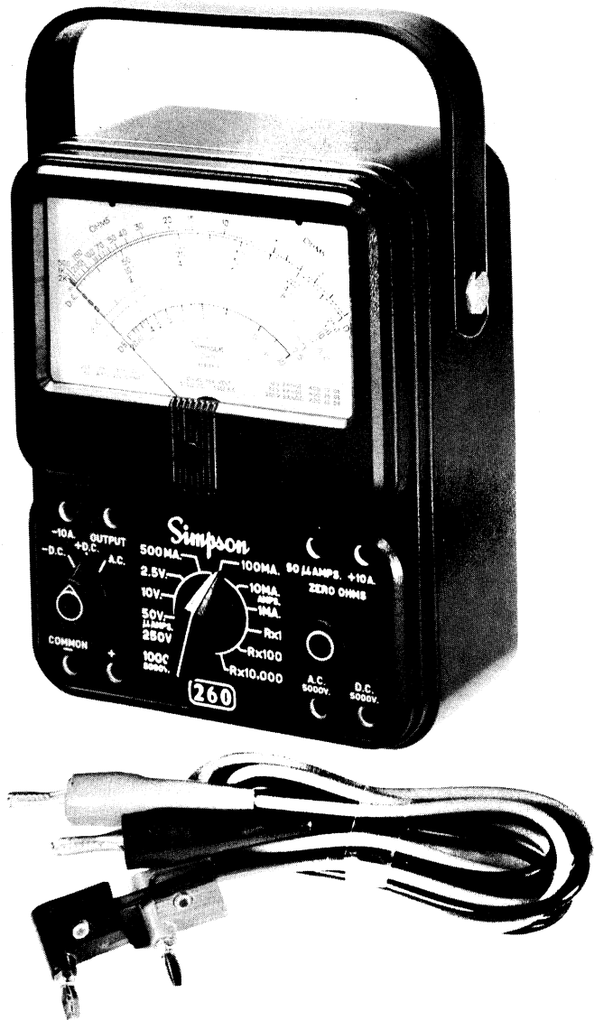
FIG. 1. SIMPSON VOLT-OHM-MILLIAMMETER MODEL 260.
