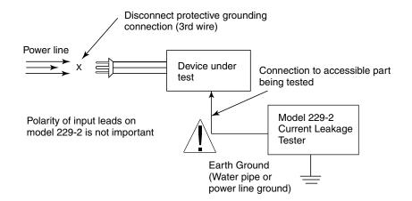
Figure 2-1. Model 229-2, Leakage Current Testing Diagram
