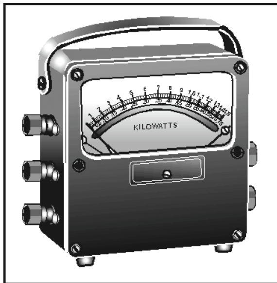
Figure 3-10.—Typical electrodynamic wattmeter.
